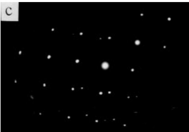
Fig. 4 TEM micrographs of double austenitized (DA) treated and 200 °C tempered steel showing dislocated lath martensite and interlath films of retained austenite. (a) Bright-field (BF) image. (b) Dark-field (DF) image. (c) Selected area diffraction pattern (SADP) from lath boundary austenite. (d) Schematic representation of (c)
